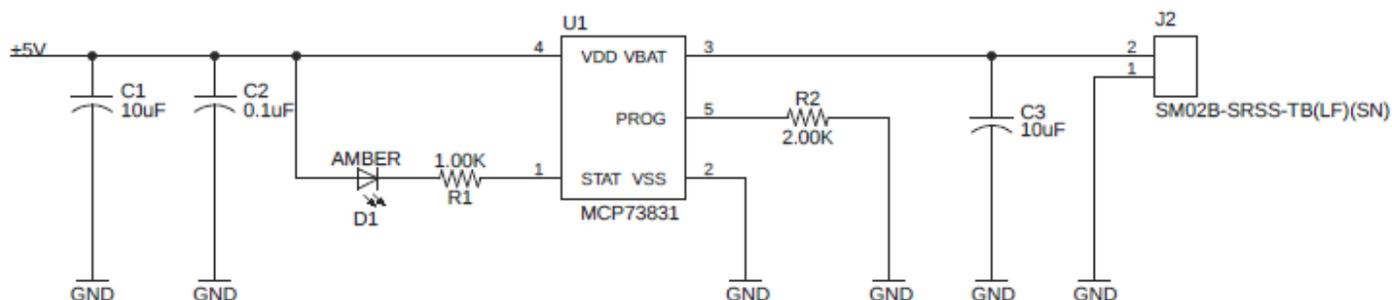
Figure 3: Sample Battery Charger Schematic
