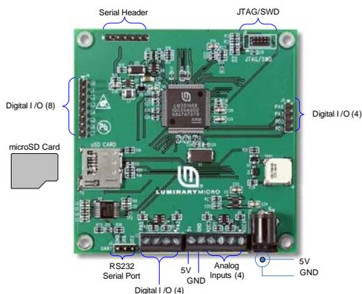
The MDL-IDM-L35 ships as a software-customizable module with the following features:
