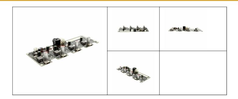
Coolgear Labs multi-port USB Type-C High powered charging circuit board is designed for integration into your own shell designs. Charge laptops, add it to a charging cart or system and experience the benefits of high power charging.
