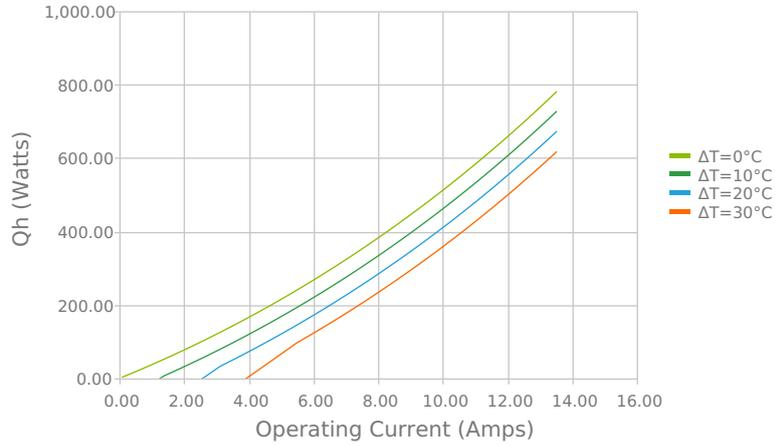
Total Heat Dissipated at Hot Side (Qh=Qc+Pin)
